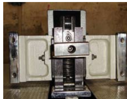
Tong of the book clamp, the lower lip of the tong should be adjustable
